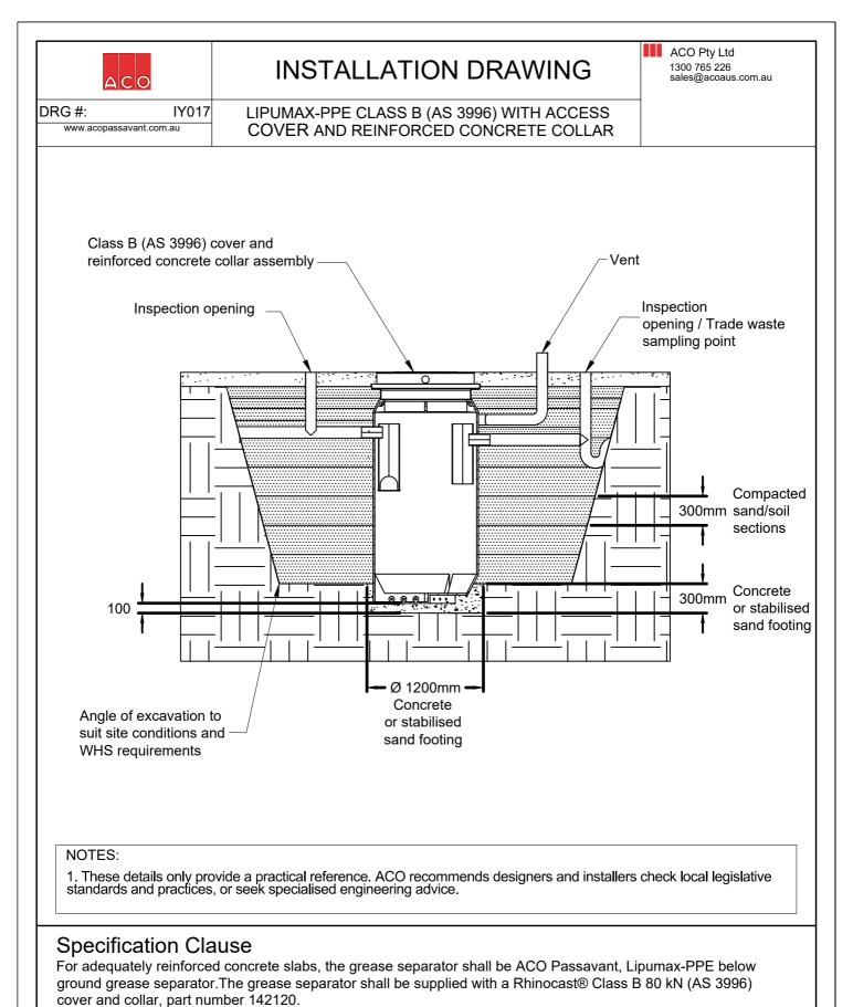
The grease separator shall be supplied and manufactured by ACO and installed in accordance with local codes and Standards.
